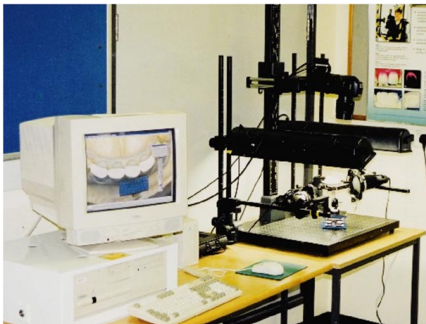
Figure 2 The image analysis equipment including a 32-bit digital camera mounted on a stand, positioned over a study model, and linked to a computer.
